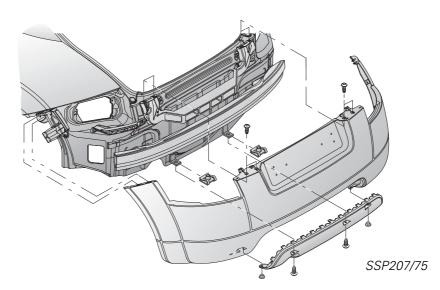
The rear bumper comprises a total of 4 parts: the bumper panel, the rear cover, the aluminium cross-member and the central locating element. The rear cover is available in two versions depending on engine variant (TT has one tailpipe, the TTS two). A seamless transition to the body side section (zero joint) is produced by means of 2 bolts on each body side section.
