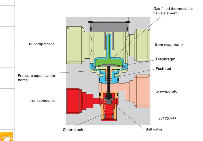
Lack of thermal insulation will lead to a change in the control characteristic setting.
