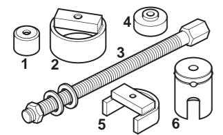
Wheel bearing puller for quattro rear axle
