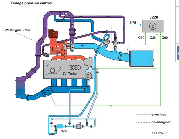
The engine control unit calculates the charge pressure setpoint from the engine torque request.
