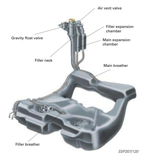
Located in the quattro fuel tank on the lefthand side is a suction jet pump which pumps the fuel from the left-hand fuel tank part upstream of the baffle housing of the fuel delivery unit.
