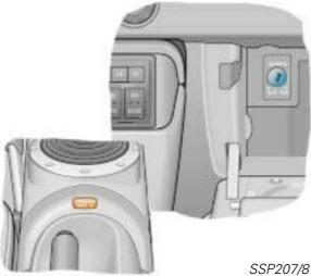
The Audi TT Coupé has a disable function for deactivating the front passenger airbag.
