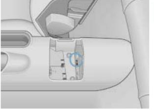
If the electrical system fails, the tailgate can be released in an emergency by means of the cable pull located below the rear central console cover.
