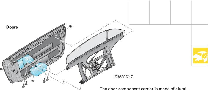
The doors of the Audi TT Coupé are frameless and of two-piece construction.
