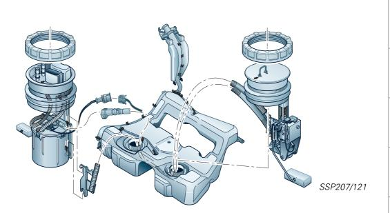
The suction jet pump is driven by the twostage fuel pump.
