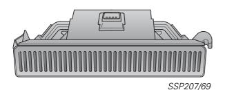
The sensor unit comprises a sender, a receiver and the evaluation electronics. The sensor unit is located behind the interior lighting in the vehicle headliner.
