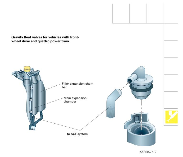
The gravity float valve prevents fuel from entering into the ACF system when cornering at high speed or if the vehicle rolls over. The filler expansion chamber as well as the main expansion chamber are combined at the filler neck upper section and purged via the gravity float valve by the ACF system.
