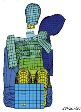
The Audi TT Coupé has head-thorax side airbags for the driver and front passenger.
