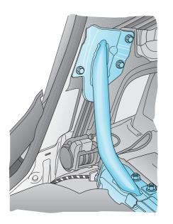
To absorb the load resulting from a side impact, the body structure is extremely rigid even though the B-pillar is not continuous. An additional transverse support extending from base of the B-pillar to the rear seat crossmember minimises cell deformation and the rate of intrusion into the side structure. This leads to low occupant loads.
