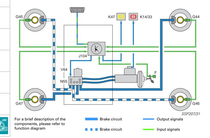
The basis of the ABS system is a dual-circuit brake system. The brake circuits are laid out diagonally and supply the front left, rear right, front right and rear left wheels. The EBPD is entirely software-supported and does not require any hardware.
