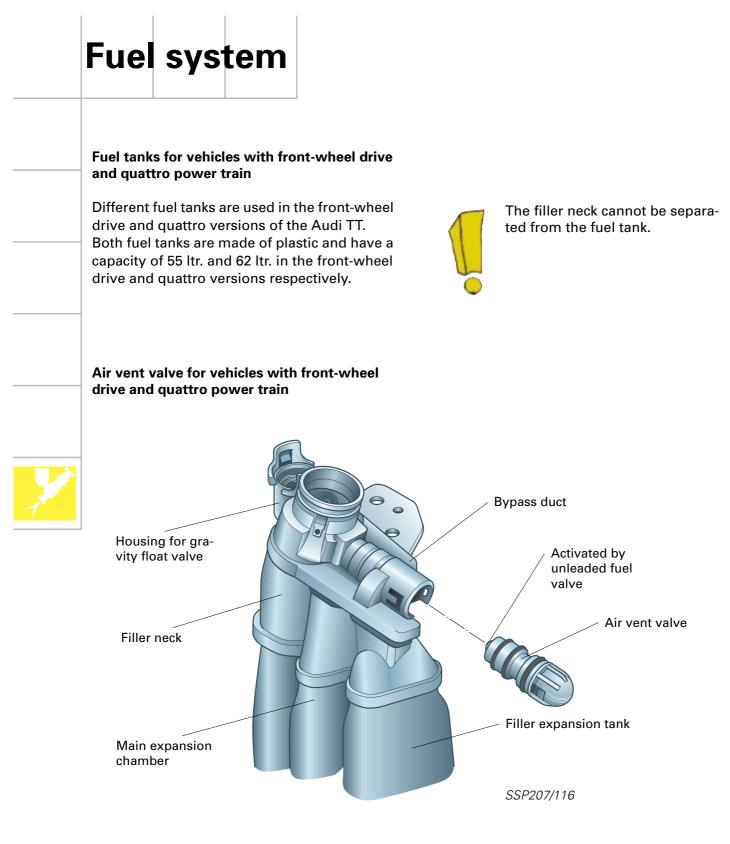
When refuelling the vehicle, the unleaded fuel valve activates the air vent valve. The valve seals the main expansion chamber so that no fuel vapour can escape from this tank when the vehicle is being refuelled.
