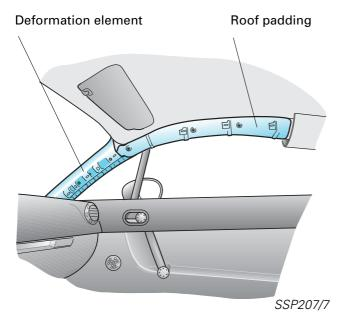
For protection of the head, a padding is also integrated in the roof area.
