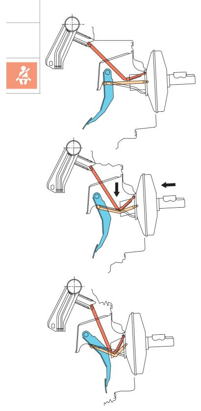
To minimise the risk of foot injuries in serious head-on collisions, the brake pedal is swung away from the foot area by means of a collapsing support if severe deformation of the vehicle occurs.
