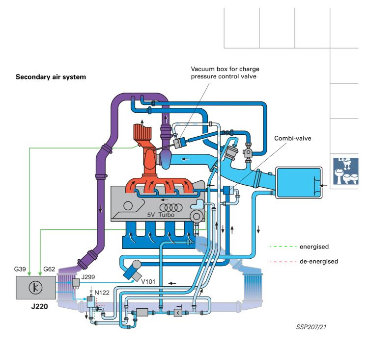
In the cold start phase, the exhaust gases contain a high proportion of uncombusted hydrocarbons.
