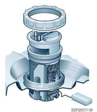
The fuel is transferred to the engine by a highperformance fuel pump with a pressure increase from 3 to 4 bar.
