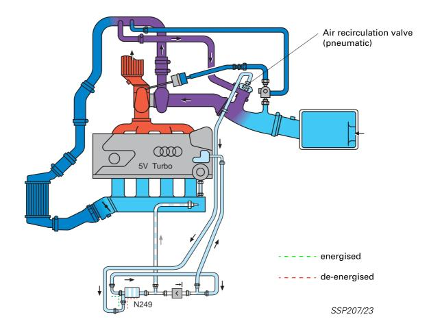
When the throttle valve is closed, it produces a backpressure in the compressor circuit due to the charge pressure still present. This causes the compressor wheel to decelerate rapidly. When the throttle valve is opened, the speed of the turbocharger must again be increased. The air divert control in overrun prevents turbo lag, which would otherwise occur.
