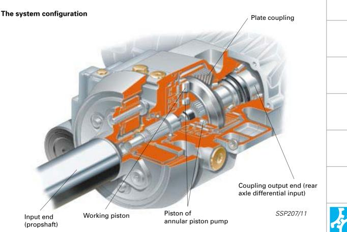
The Haldex viscous coupling is accommodated in a closed housing and mounted in front of the rear axle drive.
