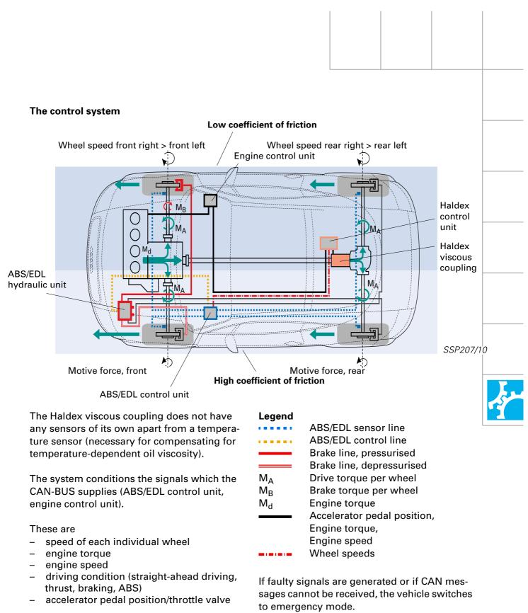
If speed signals are missing, the coupling is opened fully for safety reasons.
