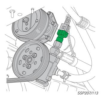
The pressure switch for power steering is located on the vane pump. It informs the engine control unit when the vane pump is subjected to a load.
