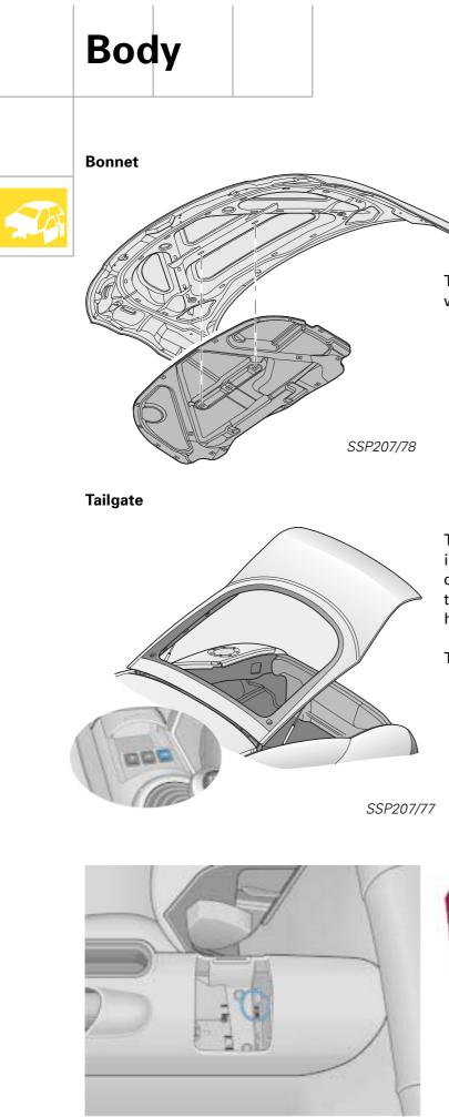
The bonnet is made of aluminium to save weight.
