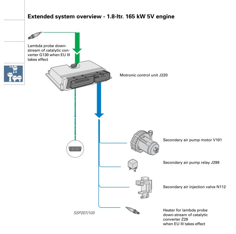
The secondary air system in the 1.8-ltr. 5V engine developing 165 kW ensures that the exhaust emissions comply with the EU III+D3 standard.
