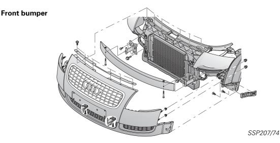
The front bumper comprises two parts: the cover panel and a decorative grille. The bumper carrier is made of aluminium and bolted to the side members by impact absorbing elements. The guide profiles attached to the left and right wings ensure an even gap all round. A zero joint is created by attaching the bumper to the wing by means of threaded bolts as well as nut and washer combinations.
