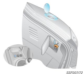
The fuel filler flap is made of aluminium. It can only be opened electrically via a switch in the central console.
